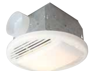
TFV50L - Builder Series Vent Trim: 12.3" Dia x 2" H Housing: 5.6" D x 7.6" W x 8.6" H 50 CFM; 3.5 Sone; 1 - 60 Watt
