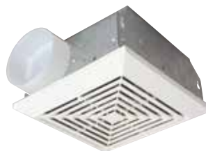
TFV70 - Builder Series Vent Trim: 8.6" D x 7.6" W x 2" H Housing: 5.6" D x 7.6" W x 8.6" H 70 CFM; 3.5 Sone
