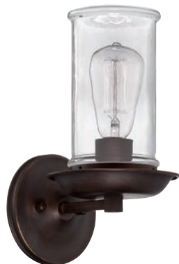
36161-ABZ - 1 Light Wall Sconce 6.13"W x 11.5"H x 7.5"E; 5.25"D Backplate 60 Watt Medium Base
