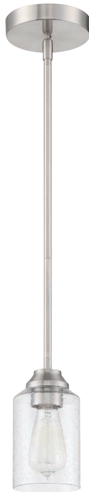
53191-BNK - 1 Light Mini Pendant 5"W x 7.75"H; 3 x 12" & 1 x 6" Downrods; 10' Wire 100 Watt Medium Base; Clear Seeded Glass - 4"D Extra 12" Downrods: Part# 531-DOWNROD-(Finish)
