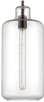
P430ESP1 - Espresso Pendant w/Rod; Clear Glass - 7.5"D 7.5"W x 16.5"H; 3 x 12" & 1 x 6" Downrod; 10' Wire 60 Watt Medium Base Extra 12" Downrods: Part# P43-DOWNROD-ESP
