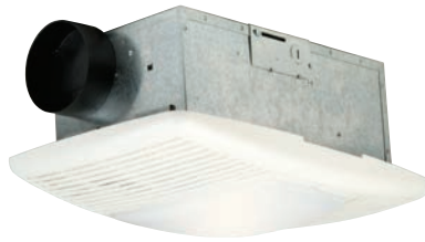
TFV70HL - Builder Series Heat Vent Trim: 12.3" Dia x 2" H Housing: 5.6" D x 7.6" W x 8.6" H 70 CFM; 3.5 Sone; 1 - 60 Watt
