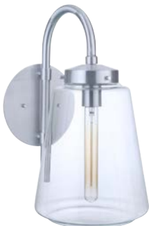
ZA3824-SA - Large Wall Mount 9.3"W x 18"H x 12.63"E; 7.48" Dia Backplate 60 Watt Medium Base; Clear Glass
