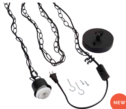
SW1004-FB - Swag Portable Pendant Hardware Kit includes 15' black chain, canopy and 15' black cloth covered plug in cord with in-line on/off switch, 2 swag hooks with wall/ceiling anchors and Black medium based bulb socket with collar. Maximum 60W bulb (not included)
