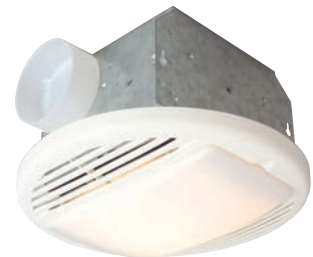
TFV70L - Builder Series Vent Trim: 12.3" Dia x 2" H Housing: 5.6" D x 7.6" W x 8.6" H 70 CFM; 3.5 Sone; 1 - 60 Watt
