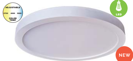
X9207-W-LED - 7" LED Pancake Flushmount Title 24, JA8, Energy Star 7"W x .7"H; Frosted Lens Cover 15 Watt LED; 1000 Lumens, 3000k, 4000k, 5000k Adjustable 90 CRI, Dimmable
