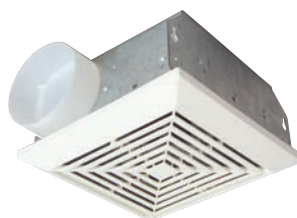
TFV70 - Builder Series Vent Trim: 8.6" D x 7.6" W x 2" H Housing: 4.1" D x 7.6" W x 8.6" H 70 CFM; 3.5 Sone
